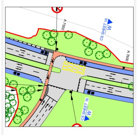
The existing three arm signalised junction is to be upgraded as per the BusConnects Preliminary Design Guidance Booklet to enhance cyclist and bus priority infrastructure. The key design rationale was to provide protected cycle infrastructure and crossing facilities, whilst improving bus priority.
