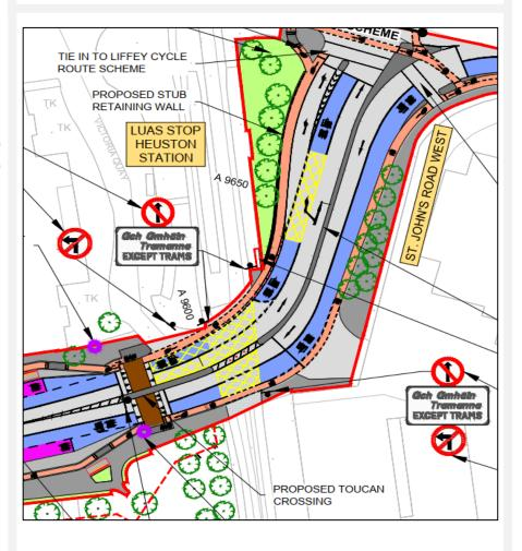
The existing signalised junction is proposed to be upgraded as per the BusConnects Preliminary Design Guidance Booklet to enhance pedestrian, cyclist and bus priority infrastructure. The key design rationale was to provide protected cycle infrastructure and crossing facilities, whilst improving bus priority and introducing more direct pedestrian crossings.
