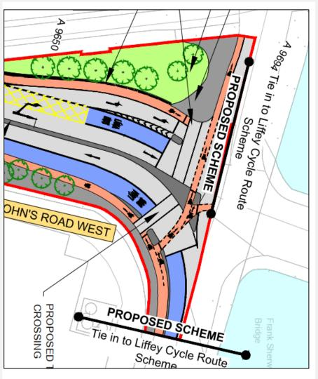
The existing 4 arm signalised junction is proposed to be upgraded as per the BusConnects Preliminary Design Guidance Booklet to enhance pedestrian, cyclist and bus priority infrastructure. The key design rationale was to provide protected cycle infrastructure and crossing facilities, improving bus priority and introduce more direct pedestrian crossings.
