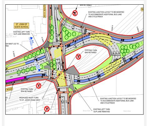
The existing major junction is proposed to be upgraded as per the BusConnects Preliminary Design Guidance Booklet to enhance pedestrian, cyclist and bus priority infrastructure. The key design rationale was to provide more compact pedestrian and cycle crossings, whilst also enhancing bus priority.
