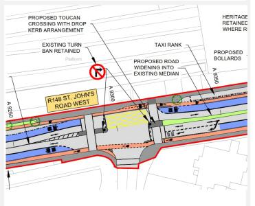
The existing 3 arm signalised junction is proposed to be upgraded as per the BusConnects Preliminary Design Guidance Booklet to enhance pedestrian, cyclist and bus priority infrastructure. The key design rationale was to provide protected cycle infrastructure and crossing facilities, whilst improving bus priority.
