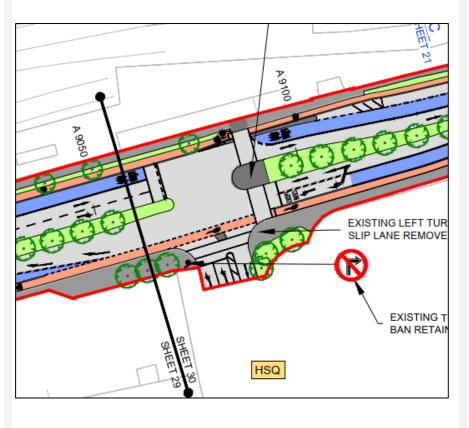
The existing 3 arm signalised junction is proposed to be upgraded as per the BusConnects Preliminary Design Guidance Booklet to enhance pedestrian, cyclist and bus priority infrastructure. The key design rationale was to provide protected cycle infrastructure and crossing facilities, improving bus priority, removing the existing left turn slip to provide a more compact pedestrian crossing.
